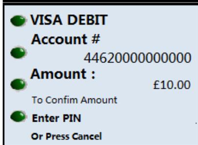
If a card was inserted into the smart card reader then the terminal will require a PIN to be entered in order to complete the transaction. Key this in and press the **Green** Enter key to continue.
