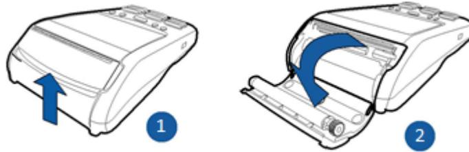
2. Remove any partial roll of paper in the printer tray by lifting it up.
