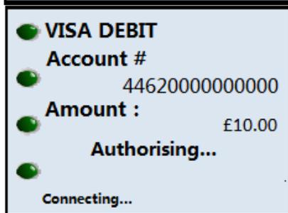
The terminal will contact the acquiring Host for an AUTH code and will display the response on the screen.
