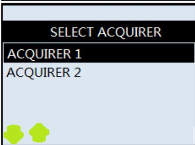
If 'One' is selected the terminal display a screen which lists all the acquirers that the terminal is configured for. Use the Up and Down arrows in the bottom left-hand corner of the screen to select the acquirer that you wish to reconcile against and press the Green Enter button.
