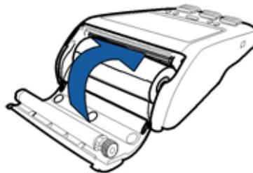
8. Tear the paper off against the serrated metal strip in the printer.
