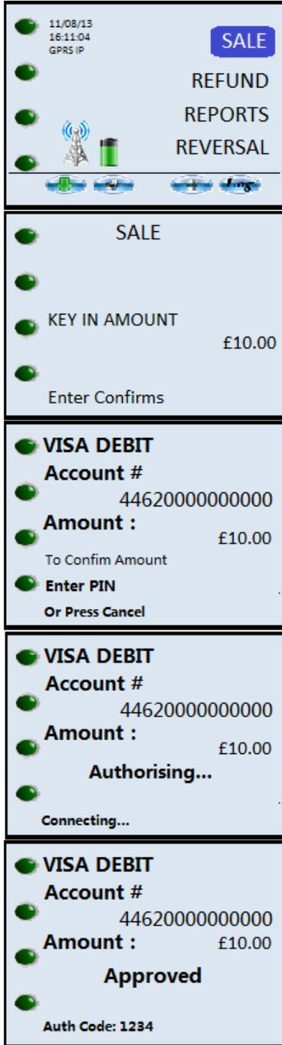
When the terminal is on the idle screen, insert the card into the smart card reader.
