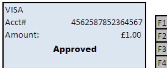
8. The terminal will contact the acquiring host for an AUTH code; the terminal will display the response on the screen.
