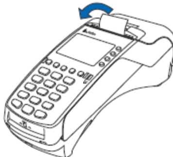
8. Tear the paper off against the serrated metal strip in the printer.
