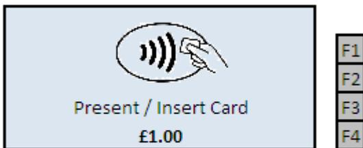
4. The terminal will prompt for the card to be presented or inserted. Insert the card into the smart card reader.
