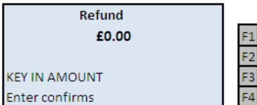
3. The terminal will prompt for the transaction value. Once the desired amount has been keyed in press the green **Enter** key. If the value entered is incorrect, use the yellow **Clear** key to amend the transaction value.
