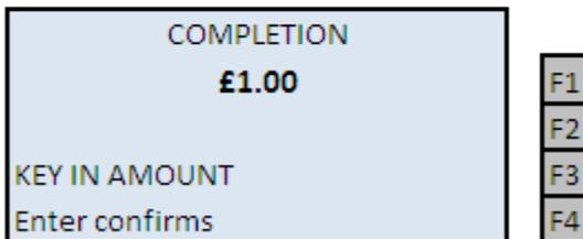
3. The terminal will prompt for the full transaction value. Key in the desired transaction value and then press the green **Enter** key to confirm. If the amount keyed is incorrect use the yellow **Clear** key to amend the transaction value.
