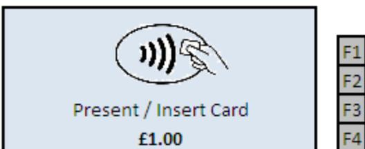
4. The terminal will prompt for the card to be presented or inserted in to the Chip reader. If the transaction value is above the ceiling limit for a Contactless transaction the terminal will prompt for the card to be inserted into the Chip Reader.
